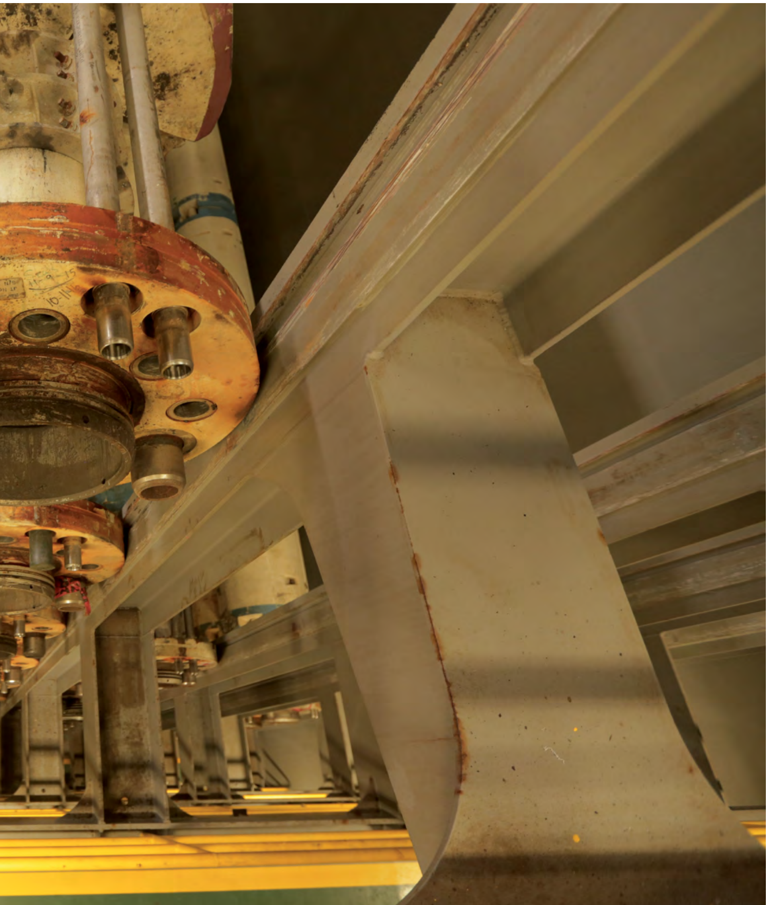
■ Casing storage on board of the Noble Bob Douglas.
